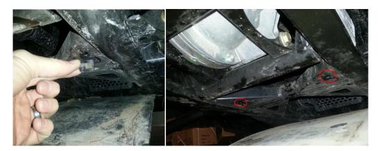
**3.** From the top side of the underbody, behind the differential you will find four holes. Place the Rear Support Bracket on top of the holes and drop (2) of the 5/16" x 2 1/2" Hex Head bolts and 5/16" flat washers down from the top as shown below. **Note: only use the front most bolt holes at this time.**
