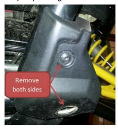
2. Remove the next four retainer bolts that hold the plastic underbody as shown in the picture below.
